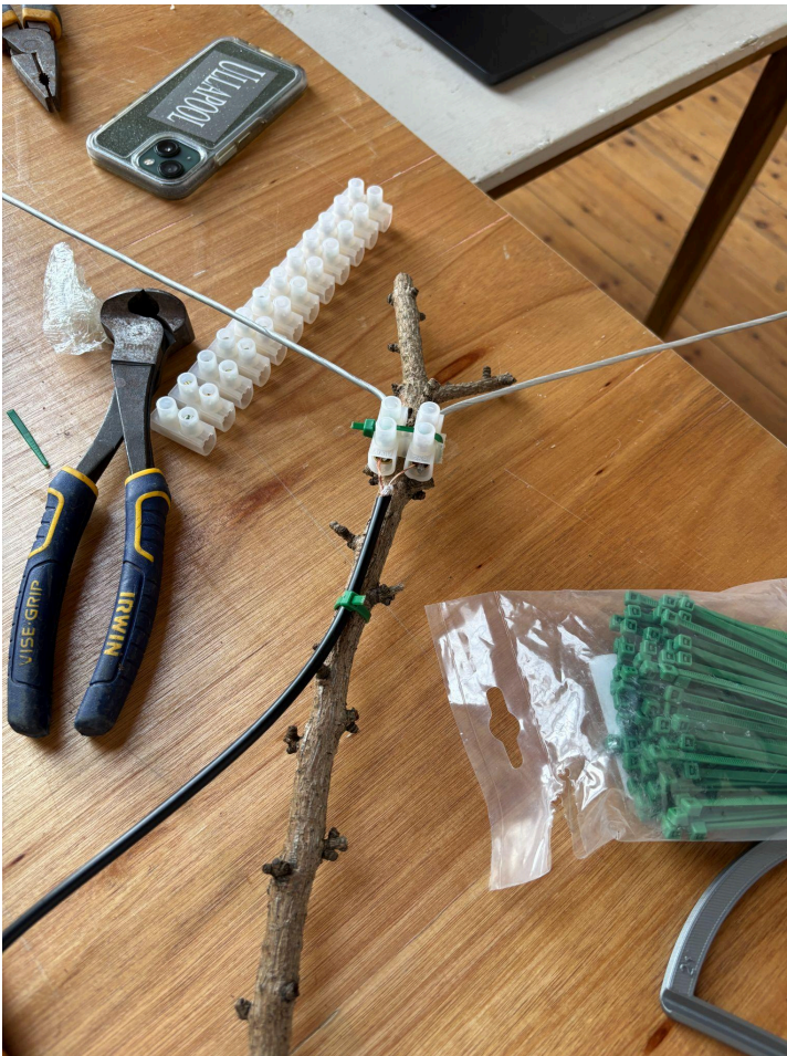
V-dipole antenna made on site by Alison and Soph.
